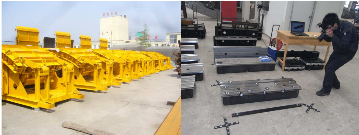
Moulds with an exterior diameter of 6000 mm for Guangzhou Subway / Photometric control of moulds by GOM
